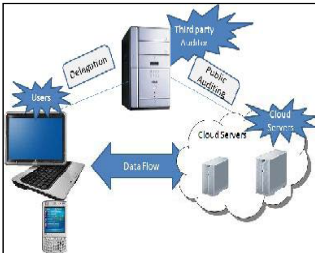
Fig 1: Cloud Storage System Architecture
