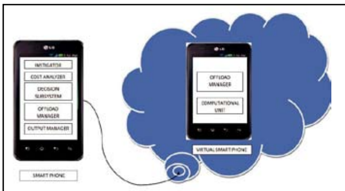
Fig. 3.: Framework of Autonomous Computation Offloading Application for Android Phones.
